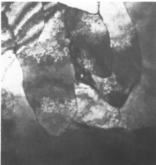
Figure 5 Typical microstructure of as-welded metal ( \times 16\,000 ).
